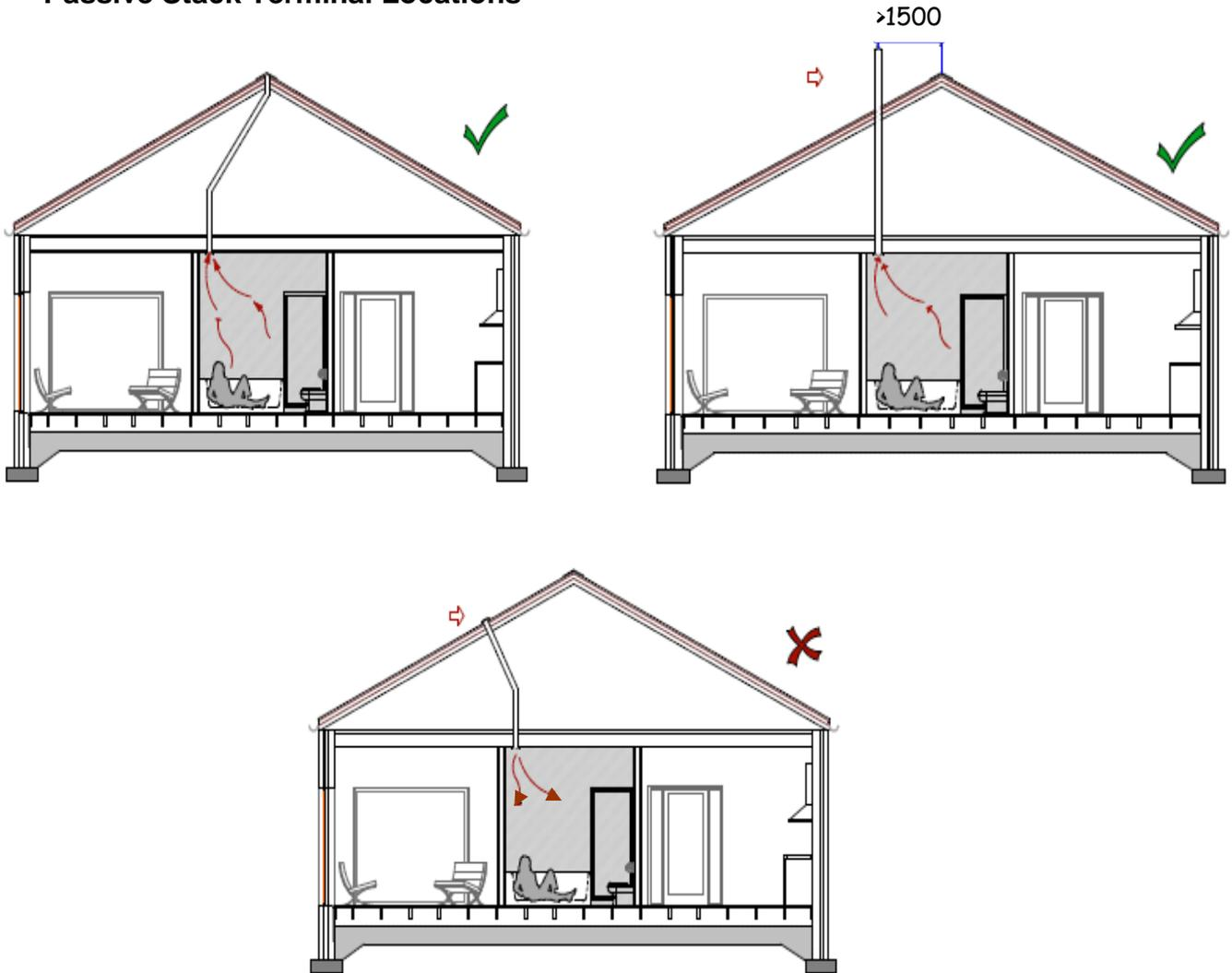
5.8 To minimise the resistance to air flow, ducts should consist of not more than one offset (i.e. not more than two bends) and these should be swept rather than sharp. Offsets should be no more than 45 degrees to the vertical.
