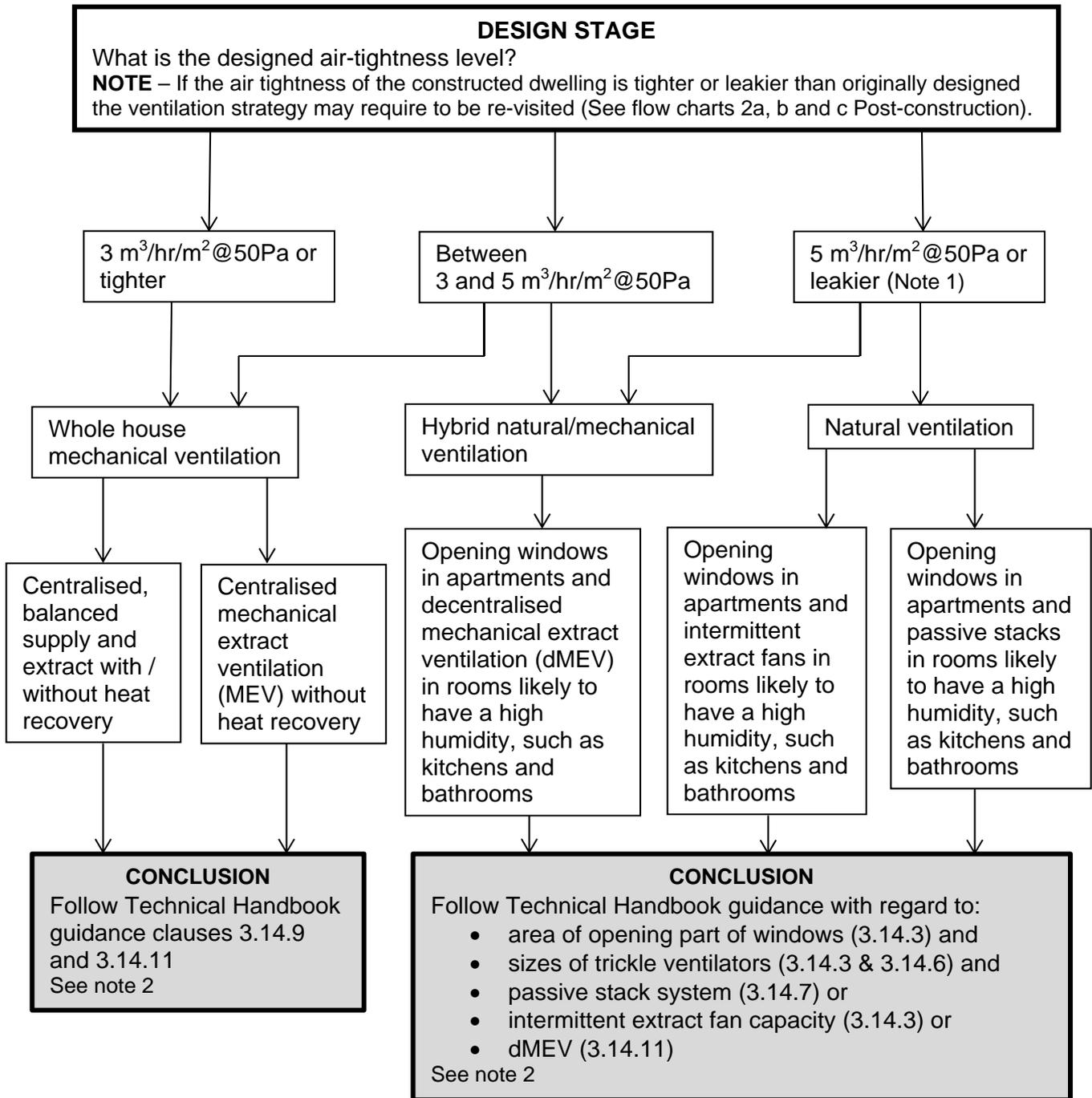
**Note 1:** Whole house mechanical ventilation is not generally suitable for dwellings with an air-tightness level leakier than 5 m<sup>3</sup>/hr/m<sup>2</sup>@50Pa.
