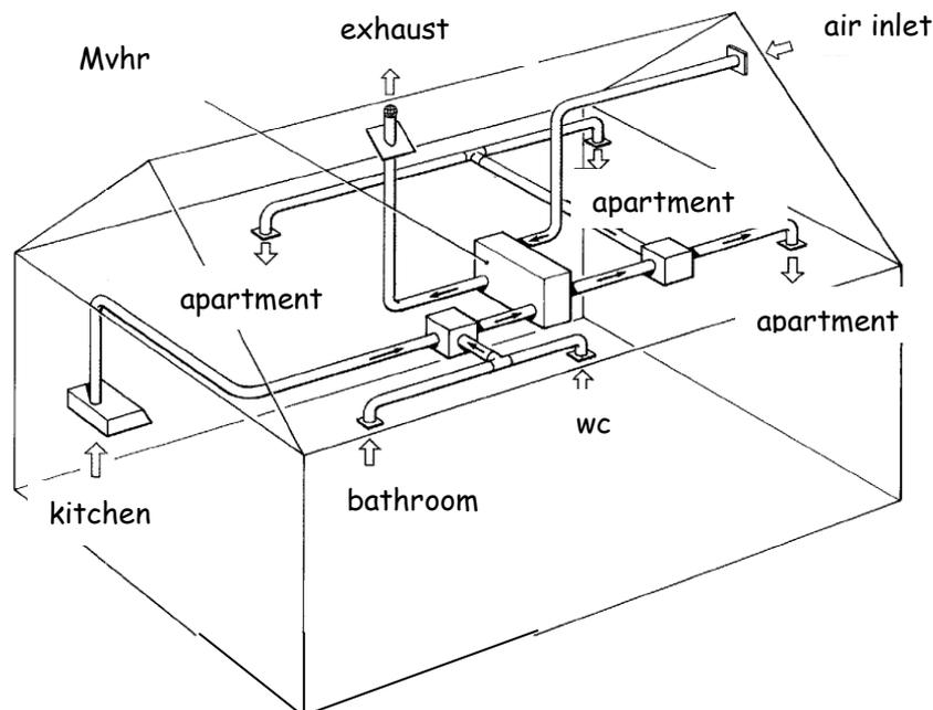
8.3 The total extract air flow rate during normal operation should be equivalent to at least 0.5 air changes per hour based on the volume of the whole dwelling. A facility to boost the air extract rate should be provided. It is preferable for a boost facility to target individual rooms rather than increase the overall extraction rate from the dwelling.
